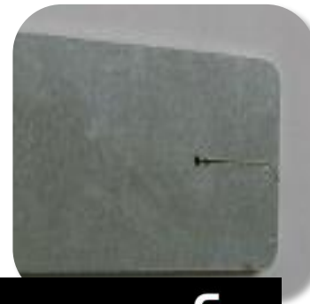
Galvanized steel @ 1000 W 1.5 mm - 15 m/min
